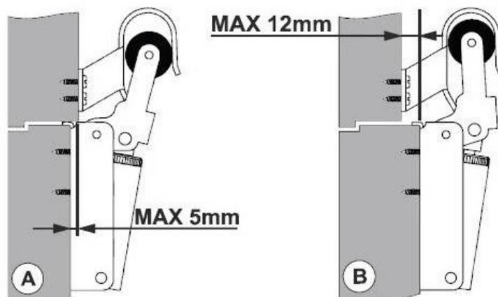
Installation limits when using the standard hook supplied with the door damper.
