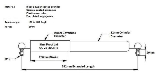
Quick and easy to install Pre-set hydraulic damping Adjustable gas closing force Opening angle: up to 110°
